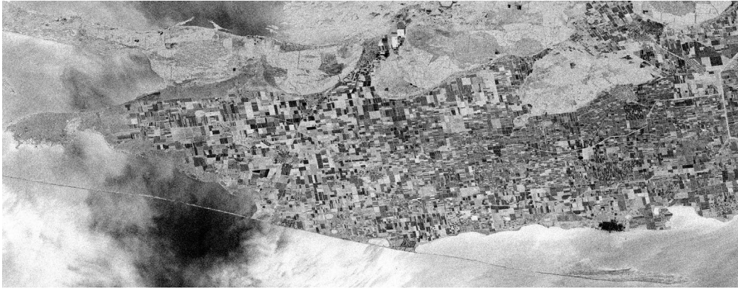
Fig. 4. The SAR-based land surface dielectric permittivity map
