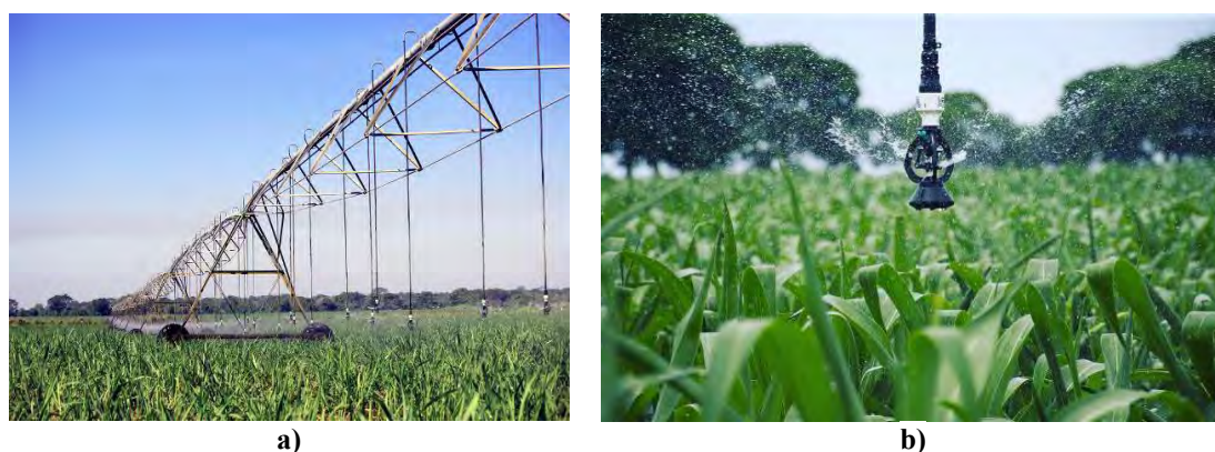
Fig. 2. Sprinkler machine [1]: a) general appearance; b) i-Wob type sprayer.
