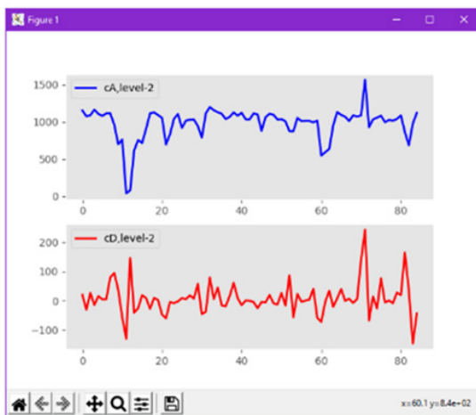
Fig. 13. The second level of decomposition of the signal into HF and LF using the Dobesha-5 wavelet
