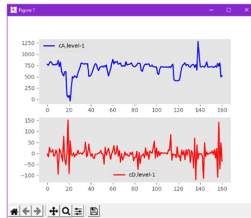
Fig. 9. The first level of signal decomposition in HF and LF using Dobsesha-5 wavelet
