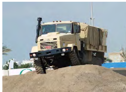
Fig. 4. Movement of a military vehicle when diagonally hung
